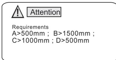
The minimum ventilation distance in diagram 1.
