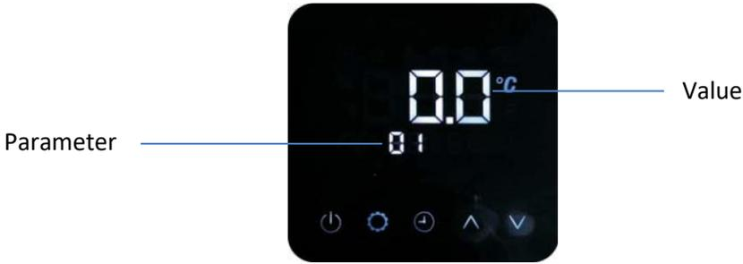
Use the UP  $\wedge$  button to scroll through the parameters. The parameters available to view are as shown below with their corresponding parameter numbers.
