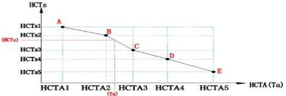
be above HCTA1, and below HCTA3. If a mistake is made when entering the values, and this is not followed, the value will automatically be corrected by the controller.
